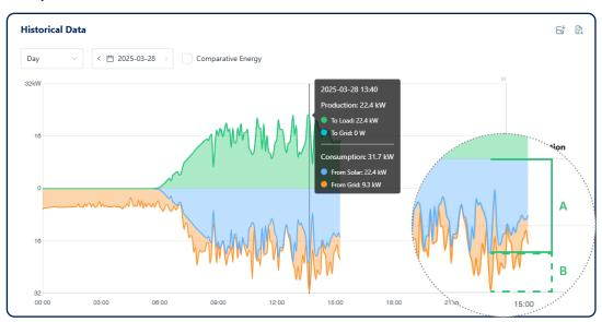
At 13:40, the total consumption (A + B) is 31.7 kW, in which 22.4 kW (A) is from the PV system, and 9.3 kW (B) from the grid.
